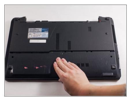
Pull down and lift up on the back panel to remove it.
