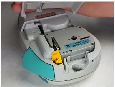
Push on the side of the cover, and pull up to remove it.
