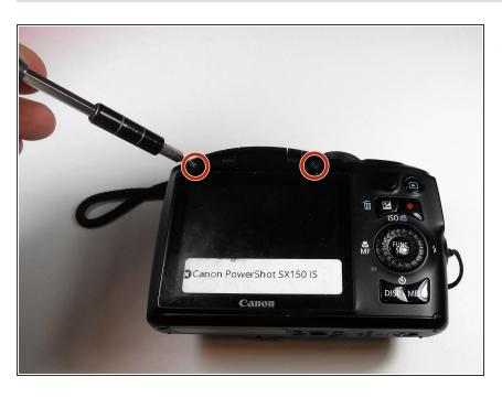
Remove the two 2mm screws above the screen using the size J000 screwdriver.
