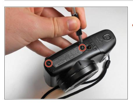
Remove two 4mm screws from the bottom of the camera with the J000 head screw driver.
