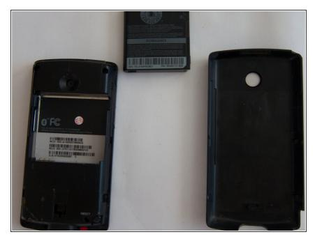
Clockwise from the top: The removed battery, the rear cover, and the phone.
