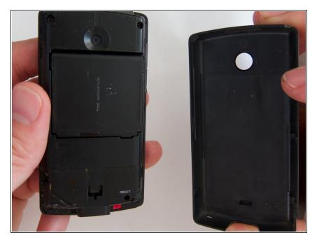
Simple photo of the back of the phone with the rear cover off.
