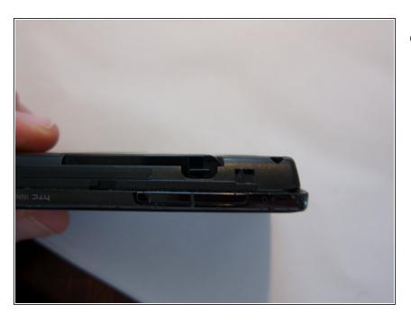
The small notch area is where the pressure to remove the battery will be applied.
