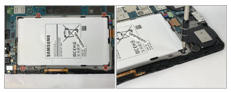
Remove the four 2.5mm Phillips #000 screws.
