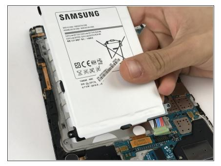
• The battery should be completely disconnected and the new one can be installed.
