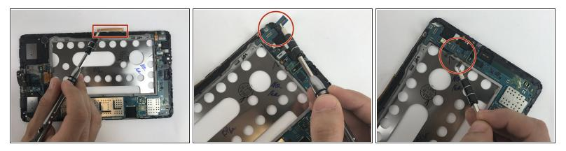
• Remove all the clips that are attached to the motherboard using your fingers or a nylon spudger.
