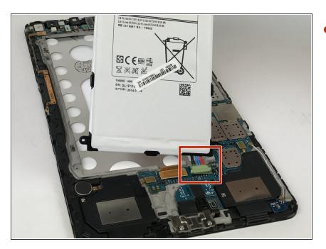
Gently pull up on the plastic tab that has red, blue and black wires that connects the battery to the motherboard.
