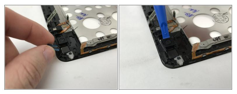
Once the motherboard has been removed, use a plastic opening tool to gently push the camera out of its place.
