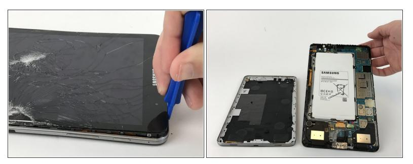
• Continue around the entire device until the back panel is completely separated from the screen.
