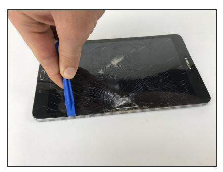
Begin by separating the back panel from the screen glass assembly using the plastic opening tool.
