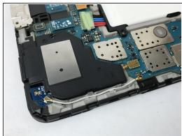
Use a Phillips #000 screwdriver to remove the 2.5mm Phillips head screw on the top part of the speaker.
