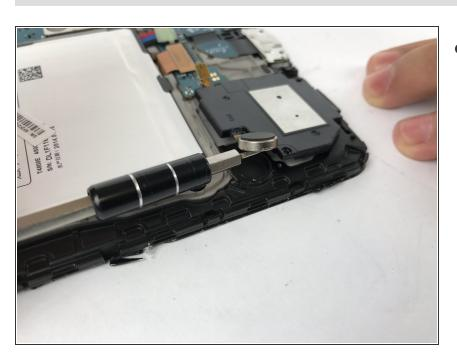
Using a nylon spudger, gently lift the round piece that connects to the speaker and remove it from its place.
