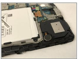
• Use a Phillips #000 screwdriver to remove the 2.5mm Phillips head screw on top of the speaker.
