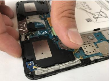
• Using your fingers, carefully remove the tab that connects the speaker to the motherboard.
