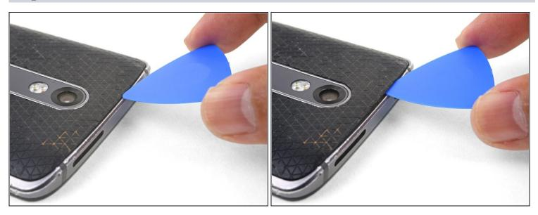
• Angle an opening pick and firmly press so that it slips under the back cover.
