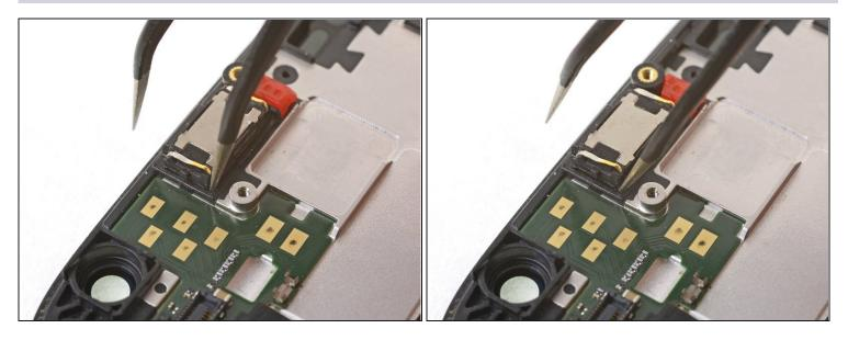
The earpiece speaker module is very delicate and prone to breaking. Be gentle when handling the module.
