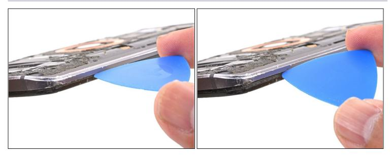
• Insert an opening pick along the frame seam and twist slightly to release the midframe from the phone.
