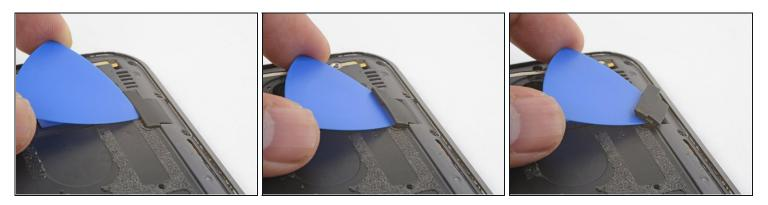
• Insert an opening pick under the flash connector rubber cover and pry forward to remove it.
