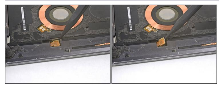
• Use the point of a spudger to pry up and disconnect the wireless charging coil connector.
