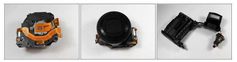
• The lens is now fully detached and can be replaced.
