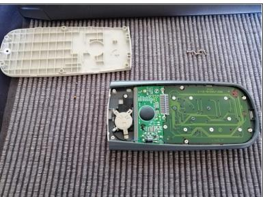
Remove the 6 screws on the back.
