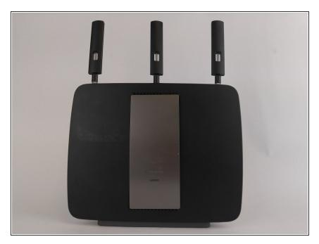
The device comes with three external antennas that use thumb screws.
