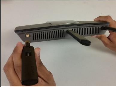
Unscrew the broken antenna using your fingers for removal.
