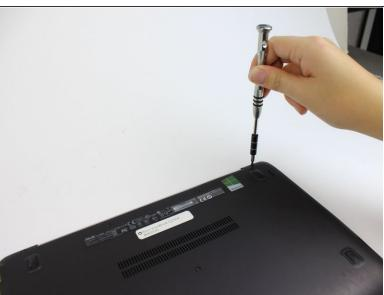
• Use a Phillips 0 screwdriver to remove nine Phillips screws from the back of the laptop (four 7mm from the top hinge, four 5mm from the bottom hinge, and one 10mm screw from the center).
