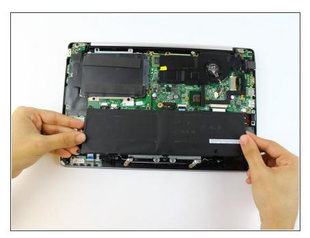
Lift and remove the battery.
