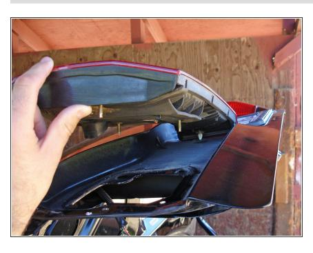
Lift the trunk tail light up from the outer edge, being careful not to break the plastic locator on the inside edge.
