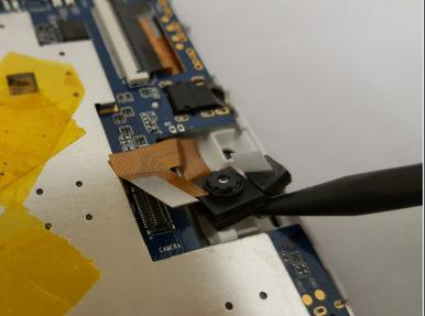
To remove the camera, simply use the pointed end of the spudger and insert it in the corner and gently lift.
