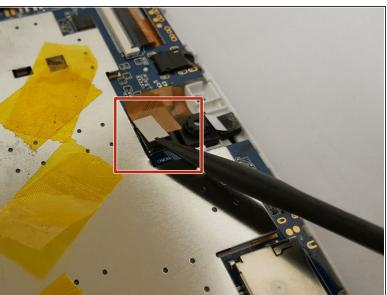
Locate the flat-top connector. Go under it with the spudger and simply lift up.
