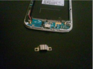
Remove clip off of USB port with a flathead screwdriver.
