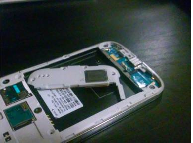
Remove Speaker using a thin rigid plastic thing, starting from where the battery nail-hold is located.
