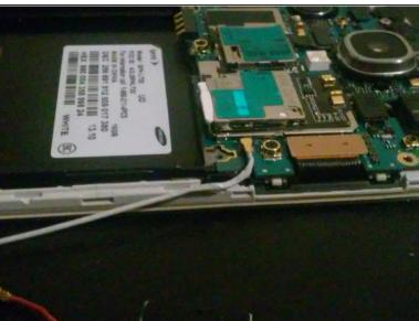
Remove the 3G and GSM antenna cable from the motherboard.
