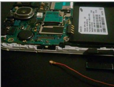
Completely remove the flex cable
