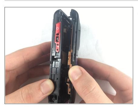
Separate the front and back casing.
