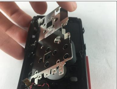
Lift the metal plate by pushing it up from the top right edge of the plate.
