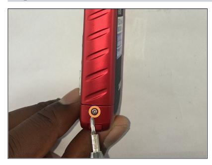
Remove the 5.00mm screw on the right of the LCD display towards the bottom of the device by using a Phillips #00 screwdriver.
