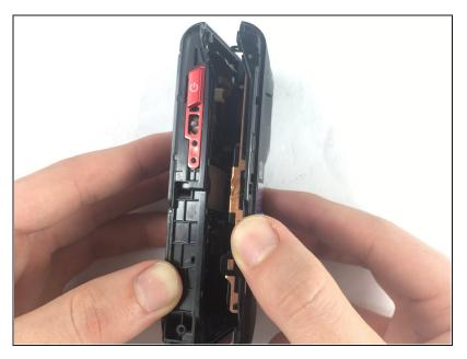
• Separate the front and back casing.
