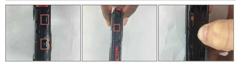
• Lift the two plastic tabs on the left side of the LCD screen and the single one on the right side on the black casing to open the device.
