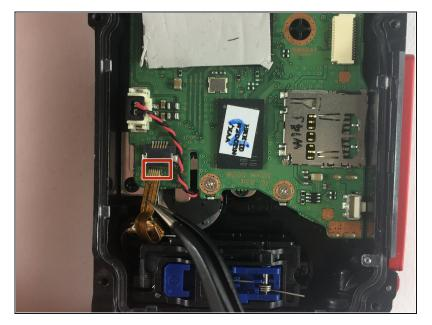
Use precision <u>tweezers</u> to gently pull out the USB connection from the motherboard.
