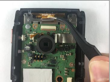
• Use precision tweezers to remove the connector joining the LCD and the motherboard.
