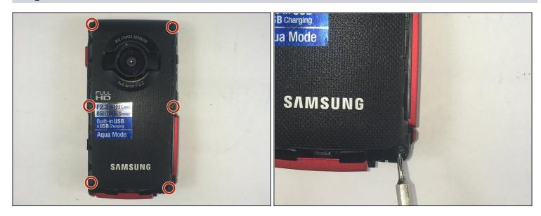
• Remove the six 5.00mm screws by using a Phillips #00 screwdriver.
