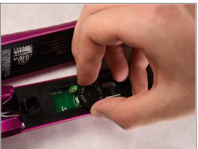
Using Philips head #00 to remove the 4 mm silver screw on the dial. Remove the dial with your hand.
