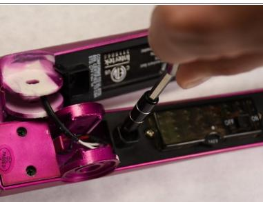
Using Philips head #1 remove the 6 mm black screw that was underneath the spring as well as the
