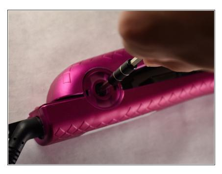
Using Philips head #2 remove the 7 mm black screw that was underneath one of the hinge covers.
