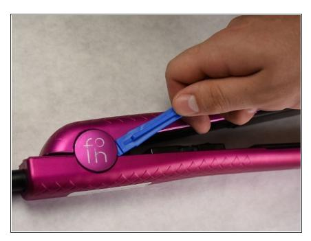
Remove both hinge covers on each side of the flat iron.
