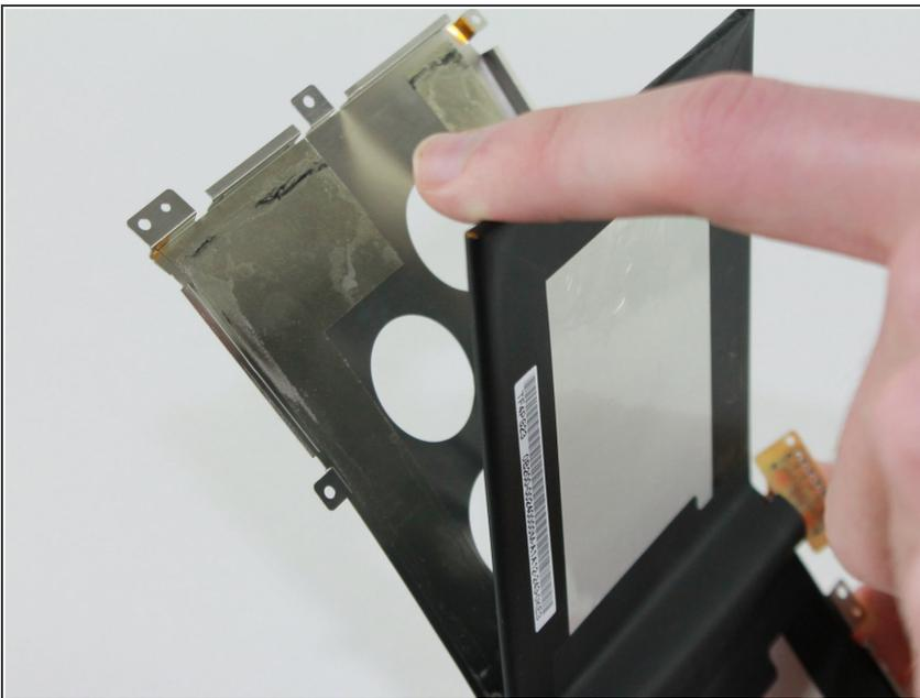
**⚠** The battery is secured to the tray by a strong adhesive. Take care not to bend the tray when removing the battery.
