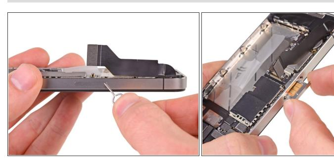
Use a SIM eject tool or a paperclip to eject the SIM and its tray.
