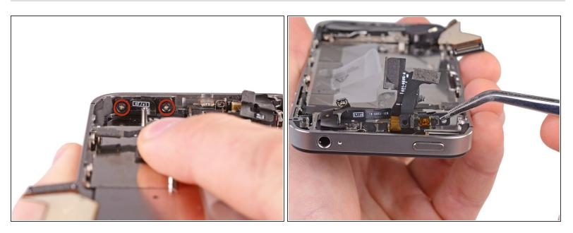
• Remove the two 1.6 mm Phillips screws securing the power button bracket to the outer case.
