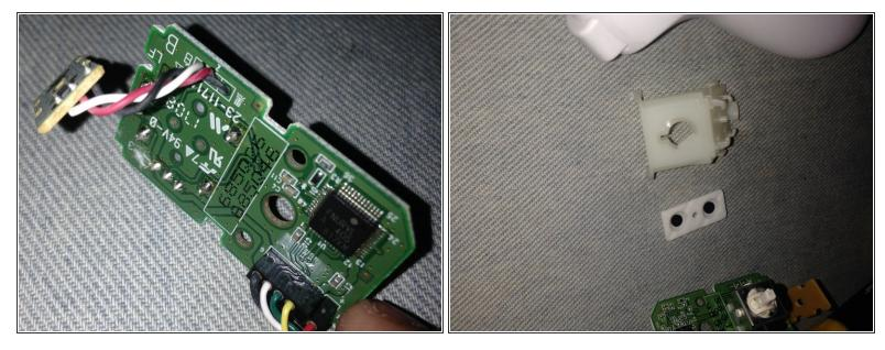
• Then remove the plastic that connects the sensor and the shoulder buttons.
