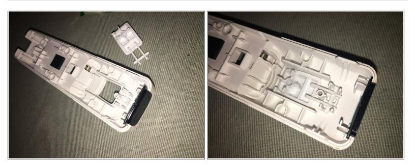
Place the B trigger back into its spot and click the two white tabs into place.
