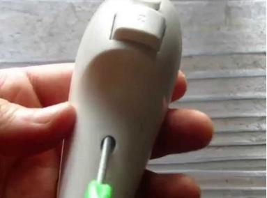
there are two small screws that need to be unscrewed on the bottom of the remote.
