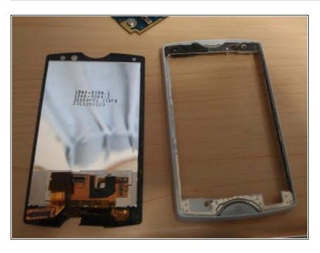
Use a thin tool to wiggle the touch screen from the metal+plastic frame, and then throw the lcd + touch
