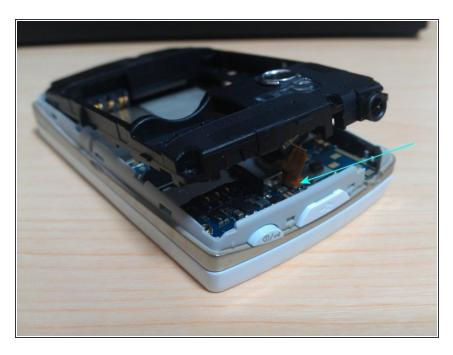
Release the Flex cable by lifting the lower end off the logic board, and lift off the back assembly.
