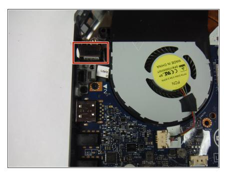
Lift up and remove the power adapter port from the computer base.
