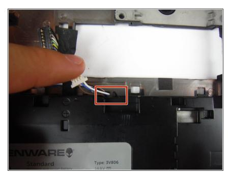
Remove the speaker cable from the cable clip on the battery.
