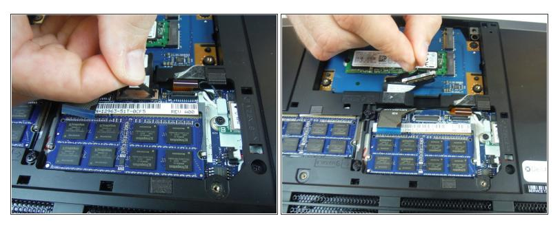
Using the pull tab, disconnect the black solid-state drive cable from the system board.
