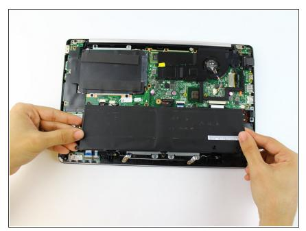
Lift and remove the battery.
