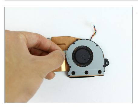
Remove the tape connected to the fan covering plate.
