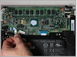
Use the spudger to press down on the 2 white port cables, while also pulling each white port cable out of their sockets.
