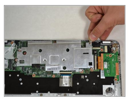
Remove the metal plate covering the motherboard by lifting it vertically.
