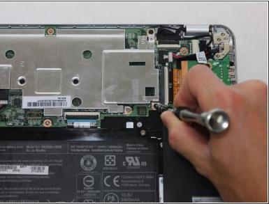
Remove the 14 Phillips 2.34mm screws using the Phillips #0 screwdriver.
