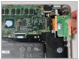
Flip up the plastic clamps holding down the 4 ribbon cables connected to the motherboard while gently pulling the ribbon cables from the sockets.
