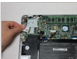
• Disconnect the motherboard from the 3 remaining cables by pulling the chords out of the sockets.
