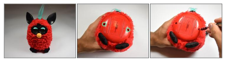
• Use a flathead screwdriver to remove the two 10mm screws on the base of the Furby.
