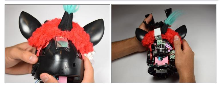
• Remove the loose, plastic back panel by pulling the panel away from Furby's body.
