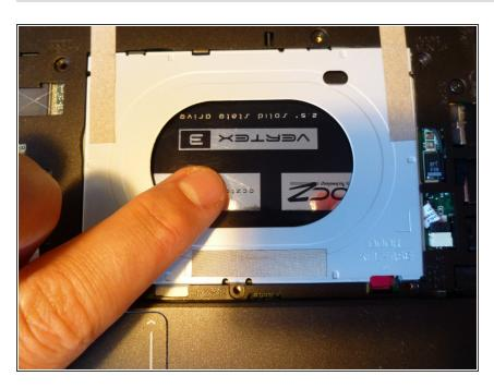
Now push the HDD downwards with the finger through the hole.
