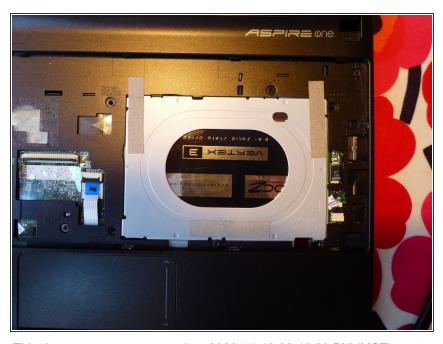
The hard disk drive is under the lighgrey casing and not screw to it.
