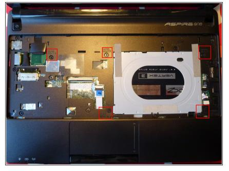
Remove the 5 screws marked with "Door".
