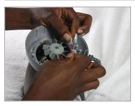
Pull off the rubber covers and separate the wires using a soldering kit.
