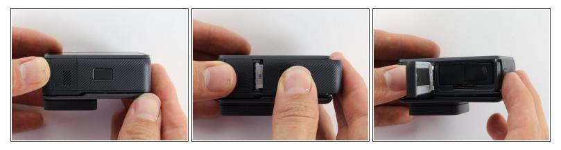
While pressing the button on the bottom of the GoPro, slide the battery door to the side to pop it open.
