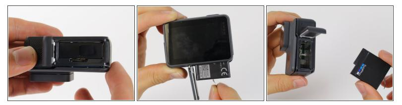
• Grab the plastic flap on the battery and pull the battery out.
