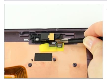
• Using tweezers, gently pull the left camera, which is the front facing camera, and small attached ribbon cable off the device and set them aside.
