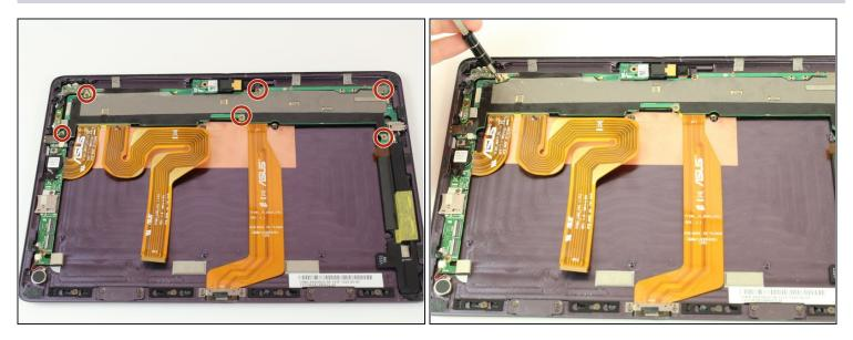
• Using a Phillips #00 screwdriver, remove the six 2.5mm screws and set them aside.
