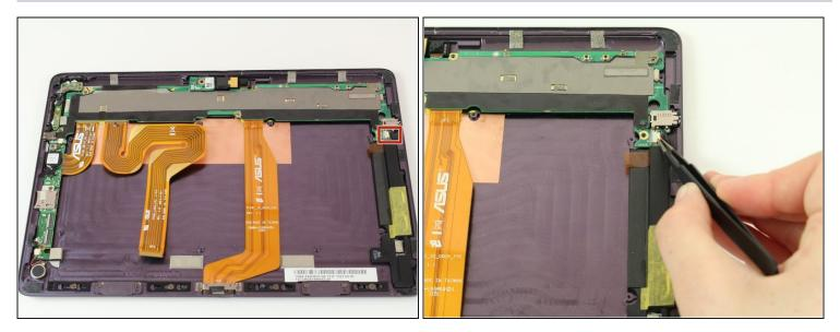
• Using <u>tweezers</u>, pull the black part of the connection between the mother board and speakers out of the white part of the connection.
