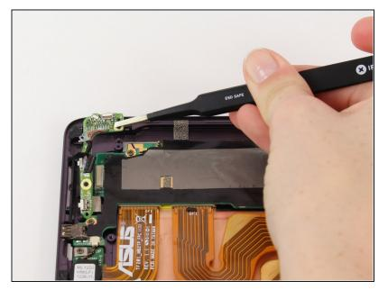
The electronic portion of the lock and volume buttons should now be free to move. Lift it gently using tweezers, and set it aside.
