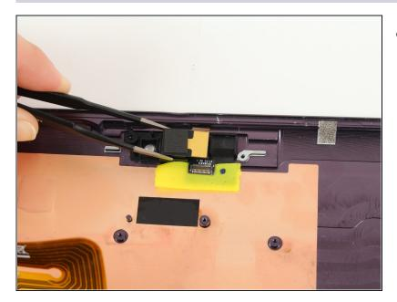
• Use tweezers to gently lift the right camera, which is the rear camera, out of the device and set it aside.
