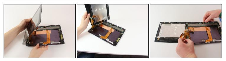
• When the screen is free of all spring clips and adhesive, slowly open the device like a clam shell with the hinge being the left hand side of the device.
