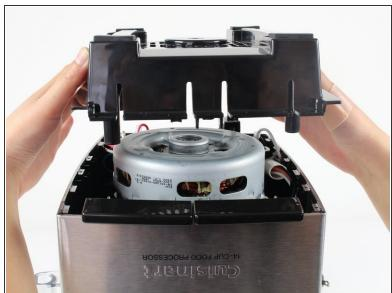
Lift off the back casing by raising it upward.
