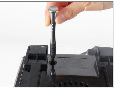
Remove the two 13.0mm screws that hold down the casing with a Phillips #2 screwdriver.
