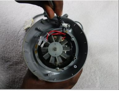
Unscrew the two 1 cm screws holding down the power cord using the #2 Phillips Head Screwdriver.
