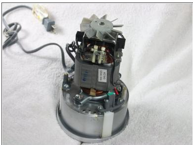
Pull off the casing from the device.
