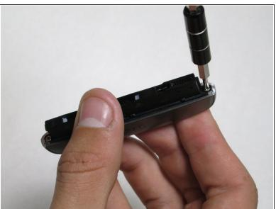
Remove the two 5.5mm Phillips #00 screws from the base of the phone.
