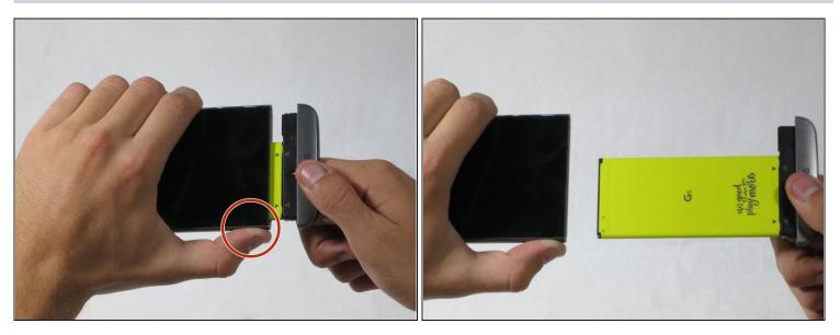
While holding the battery release button, pull the bottom end of the phone out of the body.
