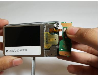
Disconnect the no-fuss ribbon cable by gently pulling it out of the button board.
