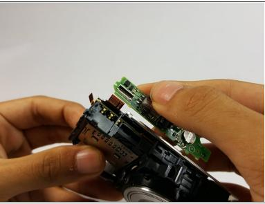
Gently pull out the no-fuss ribbon cable from the flash board.
