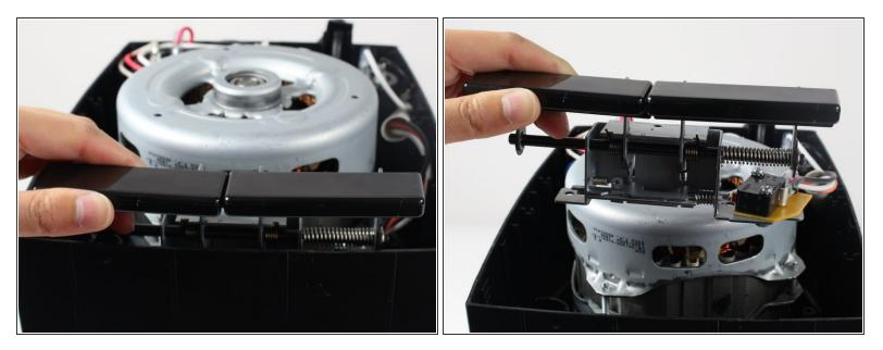
• Lift out the button assembly by pulling up.
