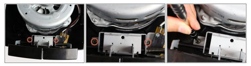
Remove the two 13.0mm screws that are holding down the button assembly using the Phillips #2 screwdriver.
