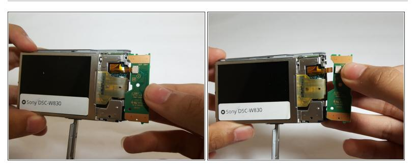
• Disconnect the no-fuss ribbon cable by gently pulling it out of the button board.
