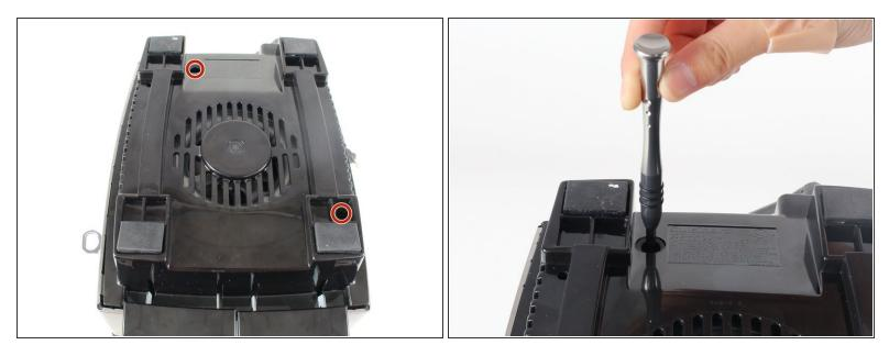
• Remove the two 13.0mm screws that hold down the casing with a Phillips #2 screwdriver.
