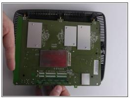
Lift the board and pull down, away from the antennas.
