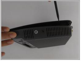
Depress the 12 clips along the edge into the router. Use the nylon spudger as using a metal object could cause damage.
