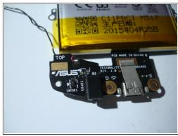
● The battery is rated at 3.85V, 11.5 Wh. The capacity is 2900 mAh minimum and 3000 mAh typical.
