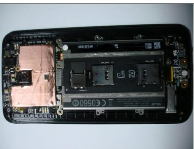
Unscrew all the 14 screws. There are two strips of adhesive running top to bottom beside the sim card slots so be patient and slowly remove the rear cover.
