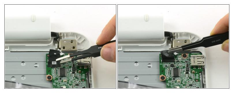
• Use tweezers to lift the fabric cover and hinge connector away from the daughterboard.
