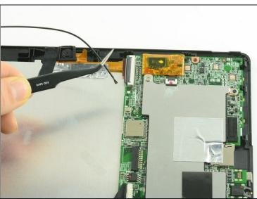
• Use ESD safe <u>tweezers</u> to disconnect the antenna from the motherboard.
