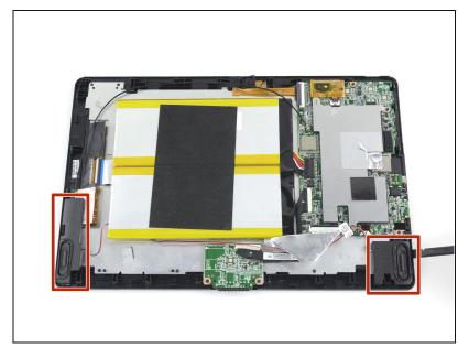
Use a spudger to lift the speakers out of the device.
