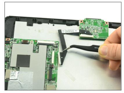
• Use <u>tweezers</u> to pull the dock connection cable away from the motherboard.
