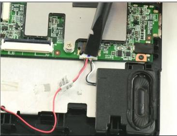
Use a spudger to release the speaker wires by pushing the bundled cabled connector away from the motherboard.
