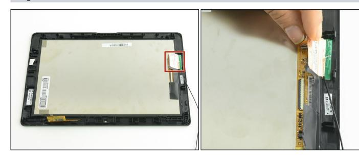
• Peel the protective flap away from the display.
