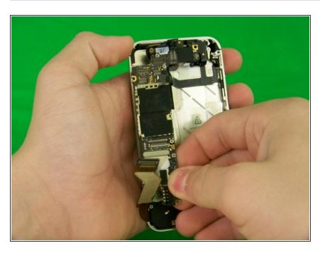
Using your fingers or a plastic opening tool carefully pull out the logic board. To reassemble your device, follow these instructions in reverse order.
