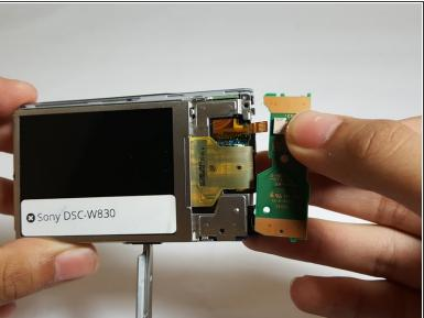
Disconnect the no-fuss ribbon cable by gently pulling it out of the button board.
