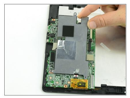
• Lift the protective shield away from the motherboard.
