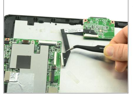
Use tweezers to pull the dock connection cable away from the motherboard.
