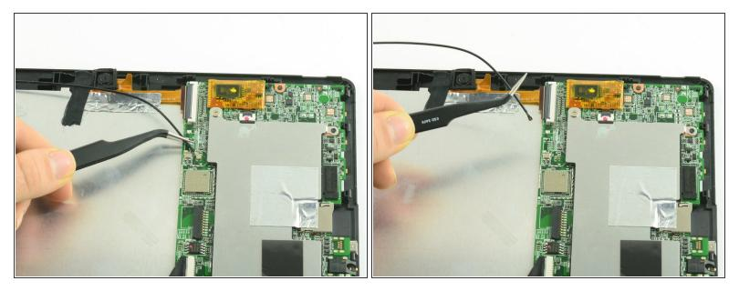
• Use ESD safe tweezers to disconnect the antenna from the motherboard.
