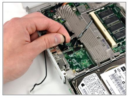
• Use the black plastic handle to disconnect the display data cable from the logic board by pulling straight up.
