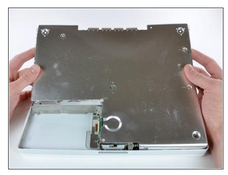
• Lift the bottom shield off.
