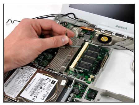
• De-route the AirPort antenna cables from the heat sink.
