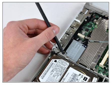
• Using a spudger, pry up the AirPort/Bluetooth board from the end closest to the hard drive. Be sure to pry against the metal framework, as shown in the picture.
