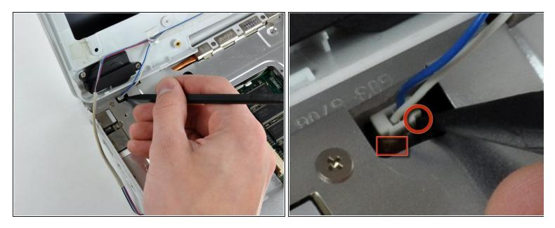
• Using the sharp end of a spudger, disconnect the connector for the blue and white power cables. Again, be careful to pry up only on the connector.
