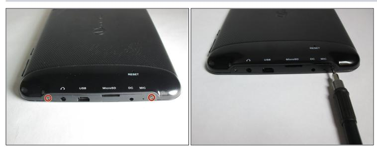
• At the bottom of the tablet, remove the two 3.6mm screws with a Phillips #000 screwdriver.
