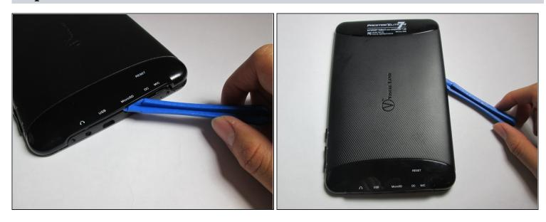
• Wedge a plastic opening tool into the edges of the tablet to pry it open.
