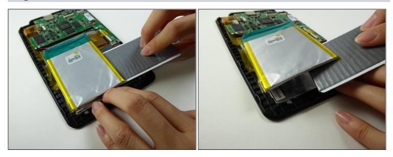
• Use a <u>plastic card</u> to loosen the battery from the tablet. Note that it will be sticky underneath the battery.
