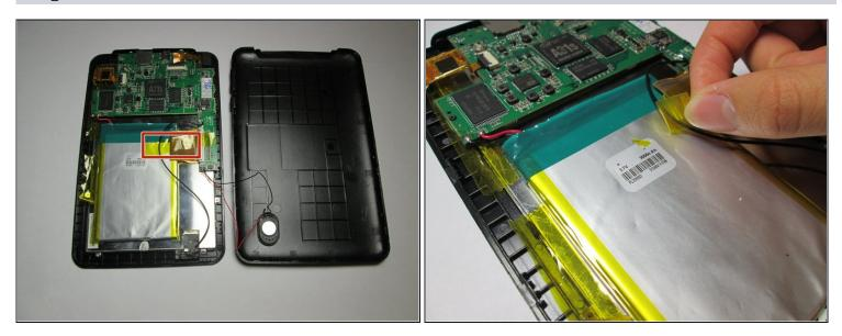
• Peel off the yellow tape holding down the battery.
