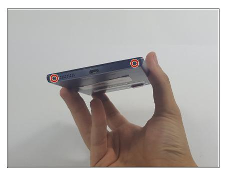
Remove the 3.65 mm Torx head screws at the bottom of the phone.
