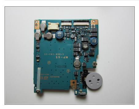
The motherboard is removed. To install the new motherboard, follow the directions in reverse.
