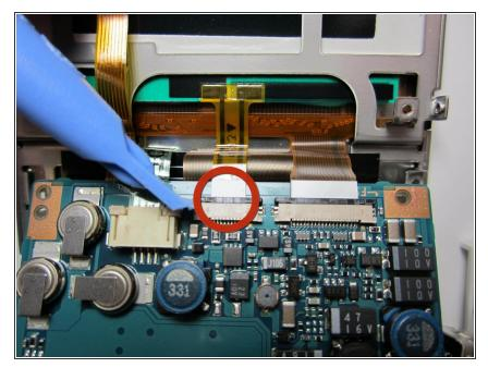
Pull out the center clip to remove the power cable.
