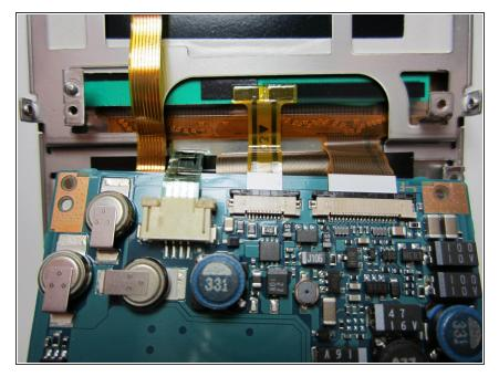
Rotate the motherboard toward you to show the cables on the opposite side of the motherboard.
