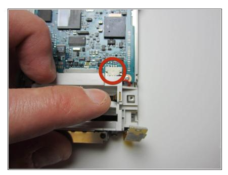
Unclip the battery harness power cable from the motherboard.
