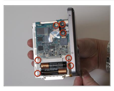
Remove the seven screws holding the motherboard to the device.
