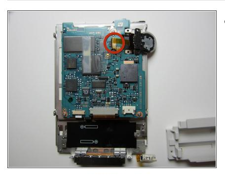
Unclip the scroll wheel power cable from the motherboard.
