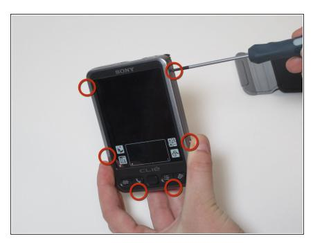
Remove the six screws holding the case together.
