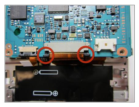
Pull out the two clips from the center to remove the power cable.
