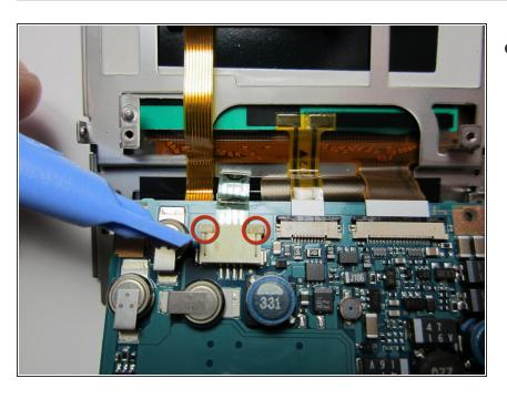
Extend both sides of the left clip to remove the power cable.
