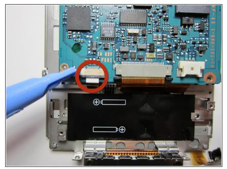
Pull the left clip to remove the cable.
