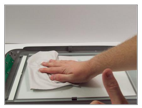
• Using a soft lint-free cloth clean the surface glass of dust, finger prints and other debris.
