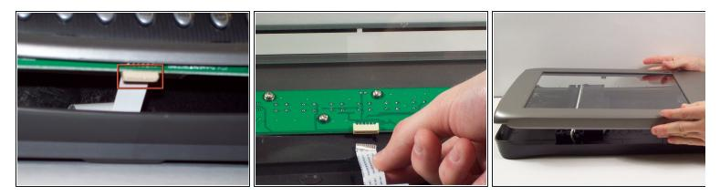
Do not fully remove the lid until you remove the ribbon cable attached to the front of the upper lid.
